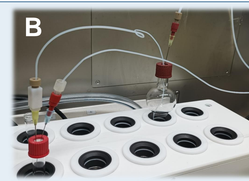
Figure 3 A & B: Xelsius ® reaction setup for optimization (left) and azeotropic drying (right)
